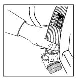
Reconnect the rear center safety belt latch plate to the mini buckle, if your vehicle has this.
